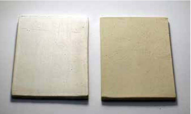
Sibelco 2502 after the bisque fire (1922°F/1050°C). Left with terra sigillata and right without terra sigillata.
